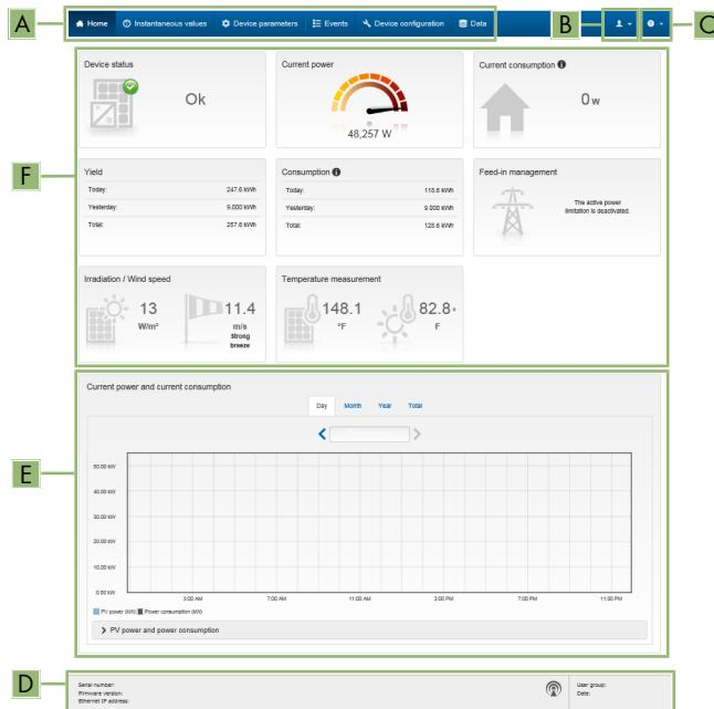
Figure 16: Design of the user interface's start page (example)
