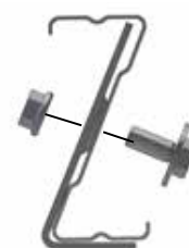
Fasten the fastening device by holding one hammer against the fastening plate and knocking in the wedge (fastening device) with a second hammer (plastic tip hammer)
